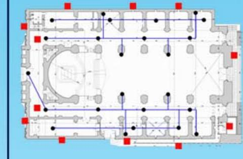
For the San Antonio Church the best solution will be the medium intensity concerning the fibre optic sensors. Because most of the damages are already visible, the sensors are only used to control them. Thats why the medium intensity concept is adequate. For the corrosion detection the high intensity concept will be used, because the salty air in combination with the wind makes harsh conditions for the building. Therefore it is nessassary to monitor as detailed as possible.
