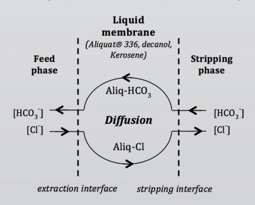
It is a membrane technology supplying substance transport between two seperated fractions using permeable membranes filled with ionic liquids. In general the chloride ions get replaced by bicarbonate ions which desalinates the water and increases its quality.
